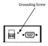
Grounding and wire router helps limit the effects of noise due to electromagnetic interference (EMI). Run the ground connection from the ground by screwing to the grounding surface before connecting devices. *Note: This product is intended to be mounted to a well-grounded mounting surface, such as a metal panel.*
